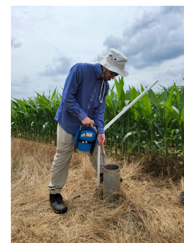
Figure 9. Static water level data collection using water level meter in Christian County, KY.
