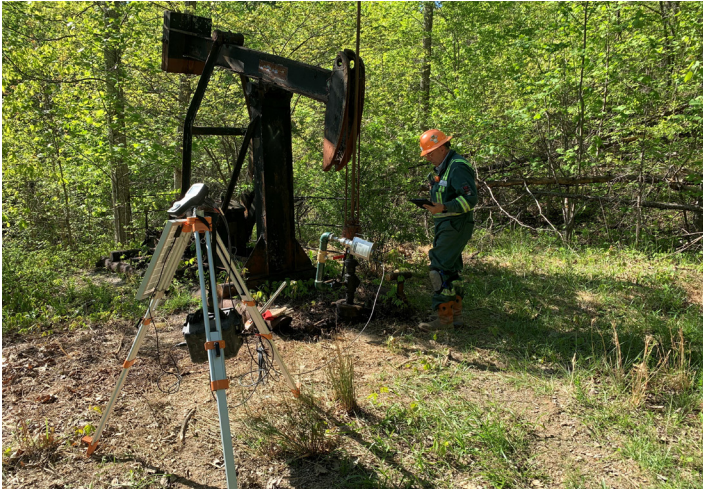
Curtis Shuck of the Well Done Foundation sets up measurements on an orphaned well in Powell County, Kentucky. Completed as a Silurian oil well on an unknown date, current methane emissions are less than 1 g/hour. Many oil wells, especially where open, are low emitters.
