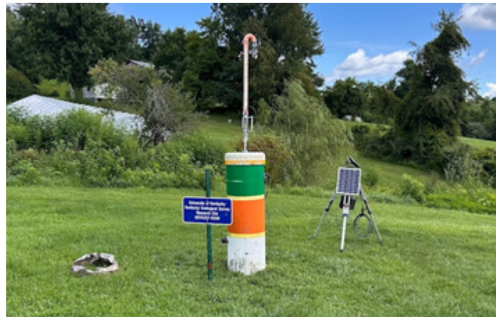
Methane measurement on an orphaned oil well in Wolfe County. The chamber with flow meter on top is located on top of 8" casing that is open at the ground surface. The well is located within 100 yards of homes and businesses. There is no completion information (date, reservoir, depth) for the well. Methane emissions for this well were less than 1 g/hour. Such low emission rates typify many open orphaned wells in Kentucky.
